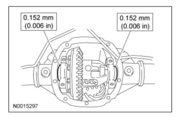
11. Using the Differential Shim Installer, fully seat the differential bearing shims. Make sure the assembly rotates freely.
